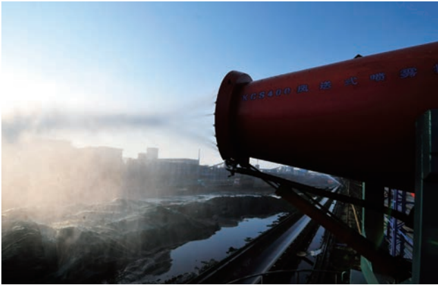
Smog gun for dust fall in coal yard
